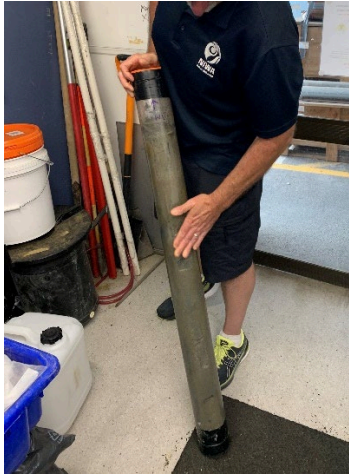
Figure 6-3: Example sediment core in the Perspex coring tube. This sample from site W1.
