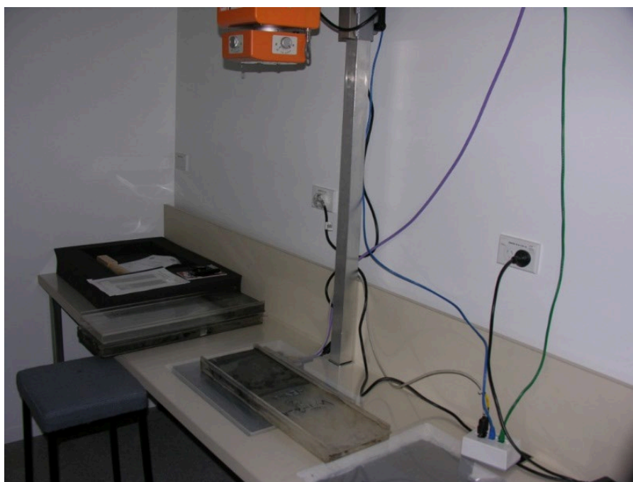
Figure 6-2: NIWA digital x-ray system with a slab mounted read for imaging. Photo: Ron Ovenden, NIWA.
