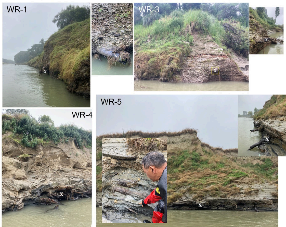
Figure 7. Wood sampled for radiocarbon dating in the lower Wairoa River. The location of each sample is marked with an 'x'. Samples WR-1, WR-3 and WR-5 were all collected from basal gravels in the river bank exposure. Sedimentology of the lower bank from which sample WR-5 was collected (horizontally-bedded clay or silt rich fine deposits, layered wood and interdigitating gravels – inset) strongly suggests an estuarine environment. Sample WR-4 was collected from wood underlying sandy alluvium at the neck of the Awamate paleochannel. Details of the radiocarbon ages are provided in Table 1.
