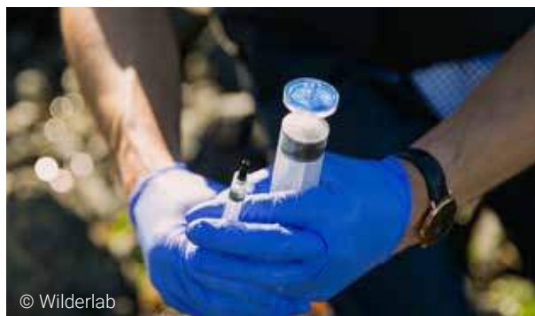
Sterile gloves are used when collecting and handling eDNA samples to avoid sample contamination.
