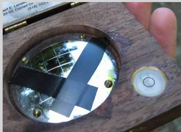
A convex densiometer with tape added to adapt for canopy closure estimates in stream environments.
