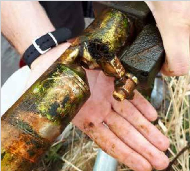
Example of biofouling on a multi-sensor meter that has been deployed in the field.
