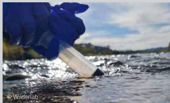
Collecting an eDNA water sample (active method).
