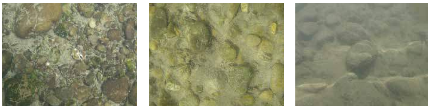
Examples of different amounts of fine deposited sediment cover. From left to right: 30%, 50% and 100%.
