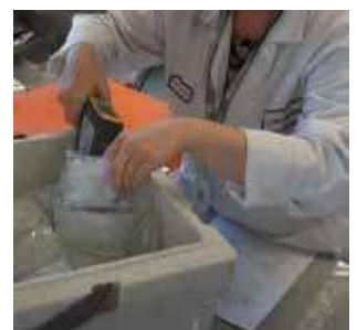
Recording arrival of samples at the lab (top) and checking the temperature inside the chilly bin.
