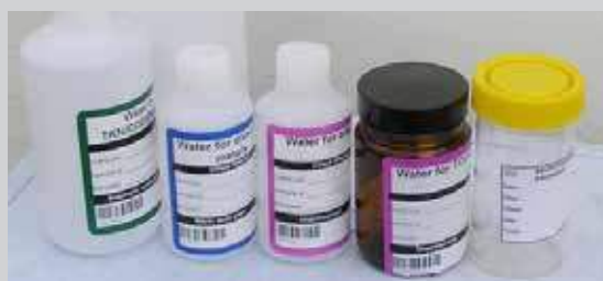
Examples of different bottles used for water sampling. The yellow top bottle is a sterile and should be filled without rinsing, with a small air gap left at the top. The green-labelled bottle contains acid preservative which will be lost if the bottle is submerged – fill this bottle from another bottle to the shoulder, cap and invert to mix.
