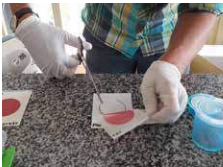
From left to right: A typical sterile sampling bottle used for collection of water samples for E. coli and enterococci testing, preparing a test plate (membrane filtration method) before incubation, checking the temperature of the water bath in a home-made portable incubator, and the E. coli colonies found on a plate after incubation. For details on colony counting, see page 96.
