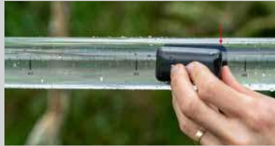
A clarity tube that comes with 1 cm increments printed along its length will make it easier to read distances.
