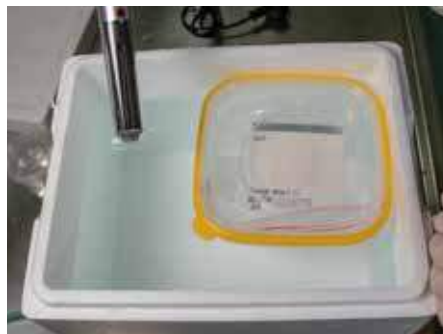
From left to right: A typical sterile sampling bottle used for collection of water samples for E. coli and enterococci testing, preparing a test plate (membrane filtration method) before incubation, checking the temperature of the water bath in a home-made portable incubator, and the E. coli colonies found on a plate after incubation. For details on colony counting, see page 96.
