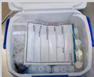
A packed chilly bin for samples destined for overnight courier delivery. Keep sample bottles upright and tightly packed to avoid movement (sometimes extra packing may be required on top). Cooler pads have been added and the Chain of Custody form is included in a zip-lock bag on top.
