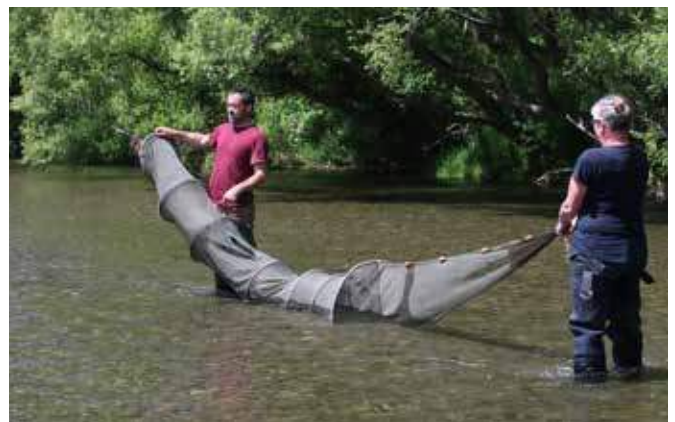
Regional council science staff demonstrating how a fyke net works. These nets should be set with the mouth facing downstream to minimise leaves and other debris from entering.
