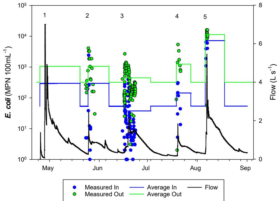
**Figure 1.** Measured inflow rate into the Toenepi wetland for the 5 events during this winter period. Measured *E. coli* in the inflow and outflow of the wetland and the averaged *E. coli* concentrations from Table 1 used in the modelling.
