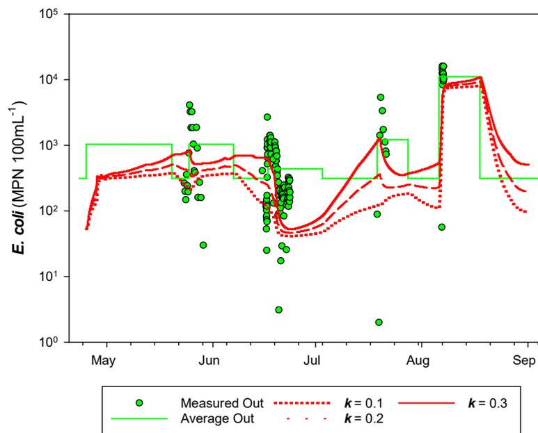
**Figure 2.** Measured and averaged *E. coli* concentrations in the wetland outlet compared to the modelled outputs using different growth rates
