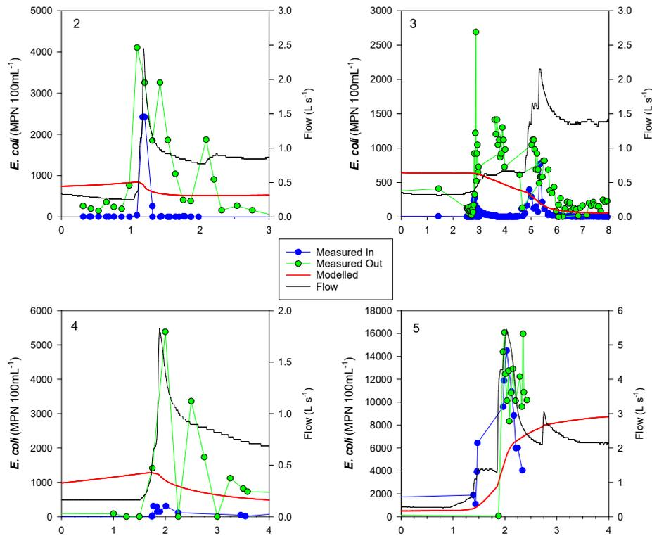
**Figure 3.** Data for individual events monitored during 2006. Shown are measured flow rates, measured *E. coli* concentrations and modelled outputs ( $k = 0.3$ ) for Events 2 to 5. The X axis scale shows days during the individual events.
