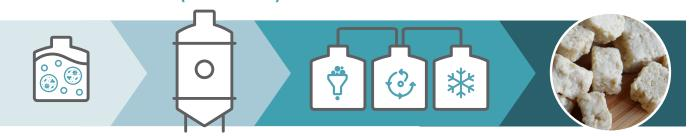
Raw materials consisting of glucose, water and nutrients are mixed and added to a bioreactor with ammonia, oxygen, and a microfungus (fusarium venenatum) that has a high protein content.
