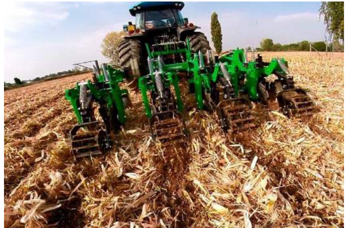
Specialised strip tillage implement. Source: sffogia.com
