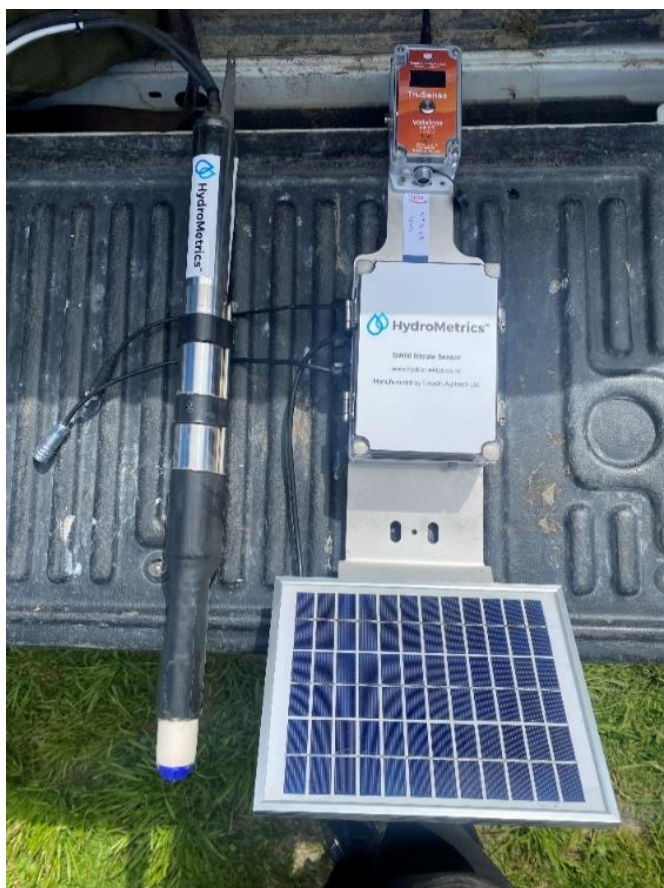
Figure 2: A Hydrometrics GW50 Nitrate Sensor
