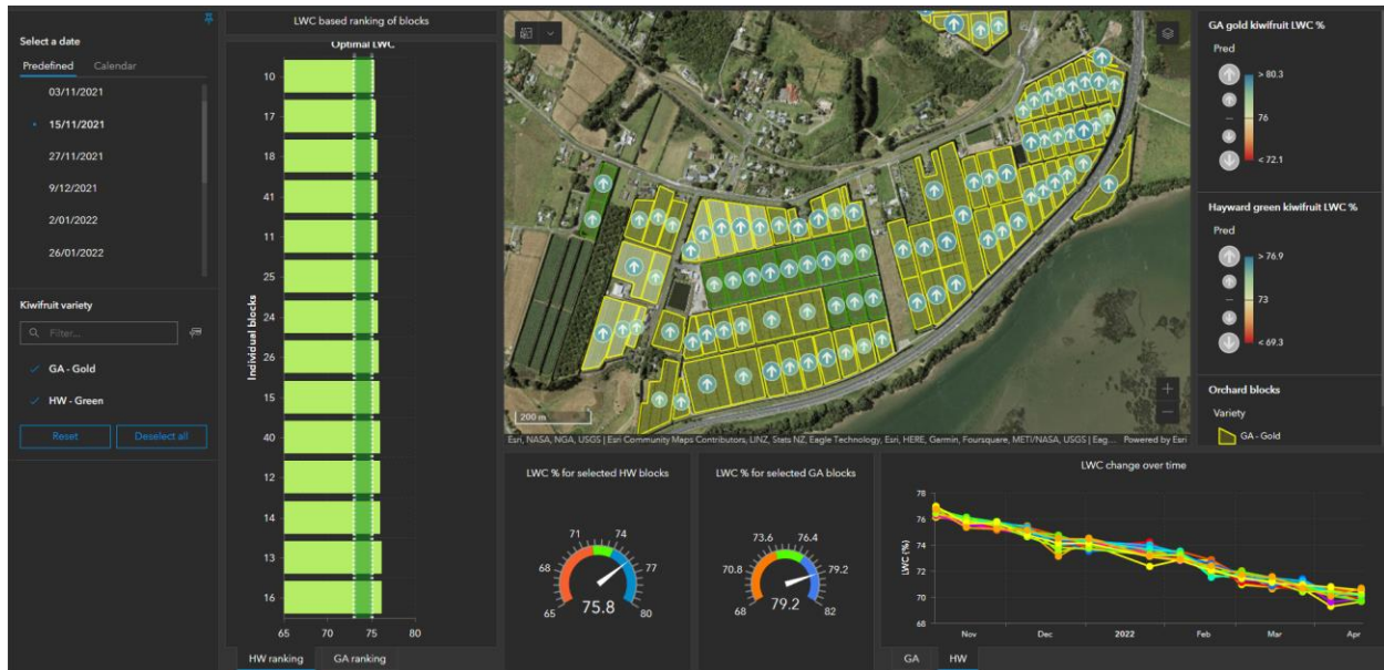
Figure 19 A snippet from the developed ESRI ArcGIS Operational Dashboard for LWC monitoring
