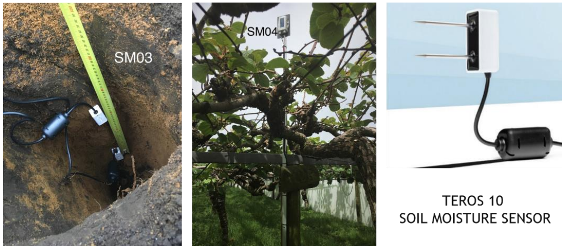
Figure 3 Installation of Teros 10 soil moisture sensors, the telemetry unit in the field and the Teros 10 sensor.
