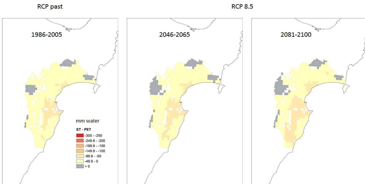
**Figure 27(continued). Mean seasonal cumulative ET - PET (an estimate of water demand; ET calculated from the Biome-BGC model ensemble average) for (1986–2005) and RCP 8.5 (2046–2065 and 2081–2100). Grey indicates that the plant water demand is met or exceeded.**
