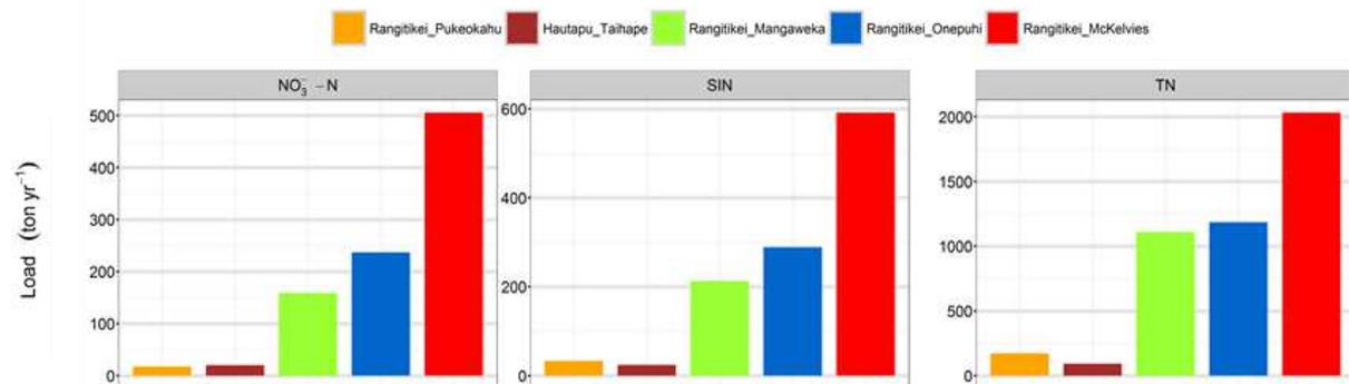
Figure 3: Estimates of cumulative average annual loads ( $\text{t yr}^{-1}$ ) of nitrate-nitrogen ( $\text{NO}_3^-$ -N), soluble inorganic nitrogen (SIN) and total nitrogen (TN) at five monitoring site in the Rangitikei River.
