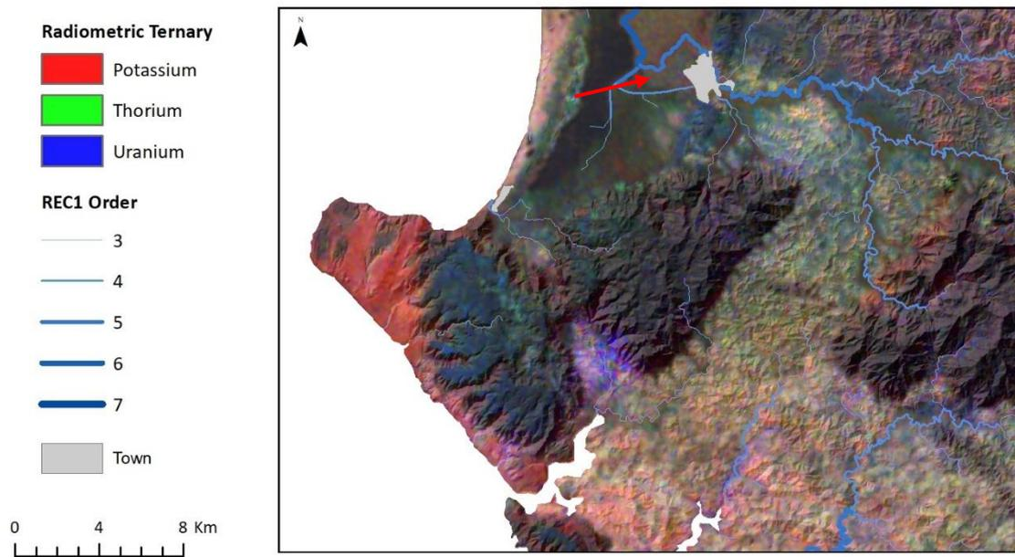
Figure 39. River order 3 and greater from REC1 and radiometric ternary at Ahipara. The red arrow indicates the Kaitaia flood plain.
