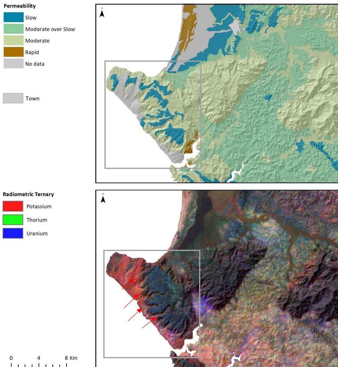
**Figure 27.** Permeability class from FSL and radiometric ternary at Ahipara. The grey rectangle outlining some of the areas with finer scale variation in landscape properties that do not appear to be well represented by the LRI. Red arrows in the radiometric ternary image denote intercalations of K-rich dune sand that has been blown along low lying valleys, which are not reflected in the LRI mapping.
