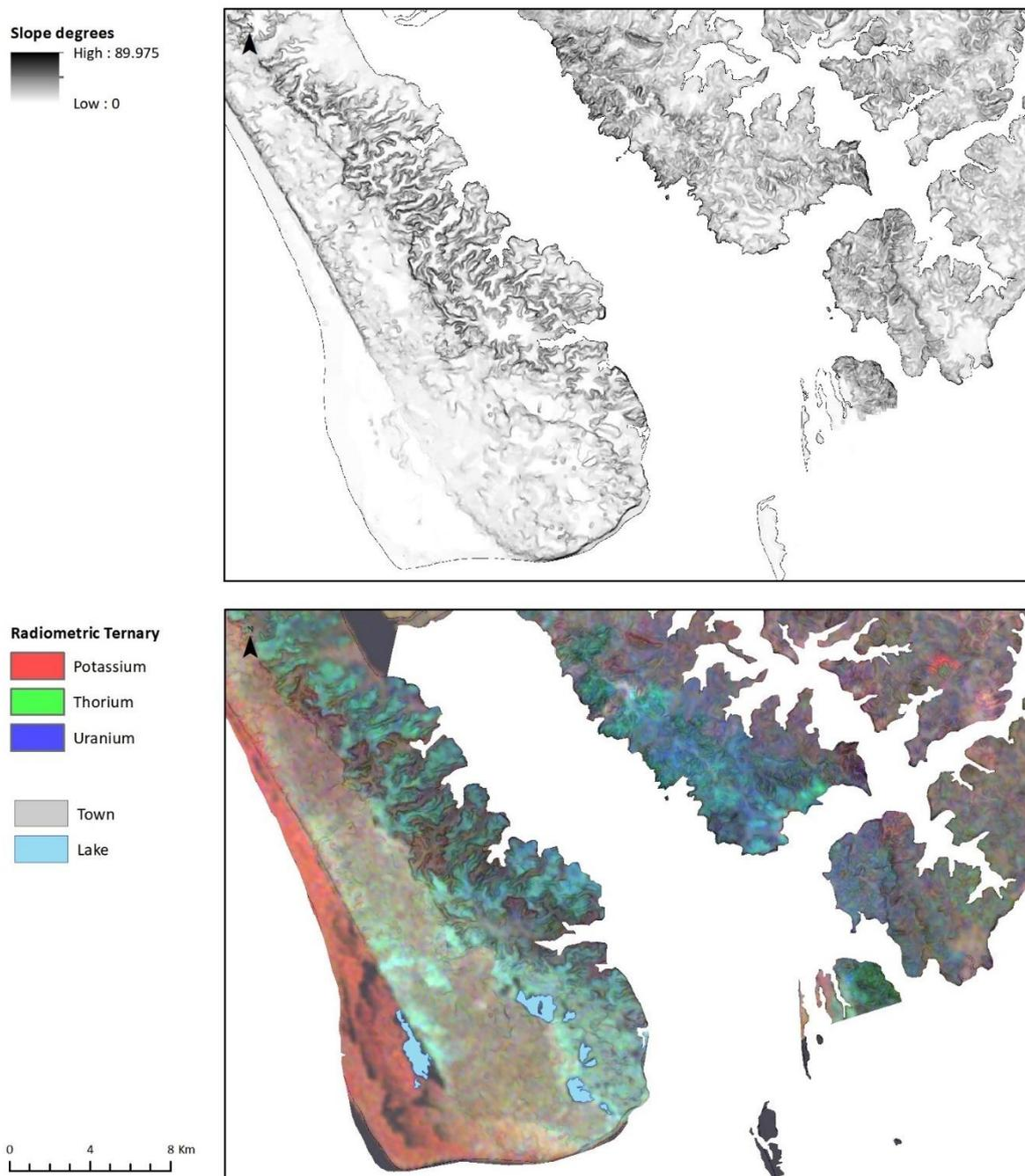
Figure 8. Kaipara test area comparison of radiometrics and DEM slope.
