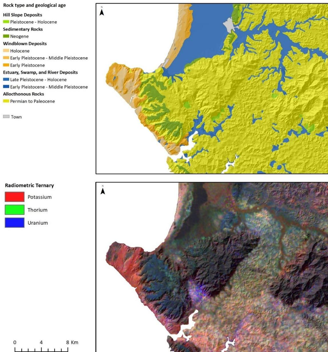
Figure 18. Rock type and age from QMAP and radiometric ternary at Ahipara.
