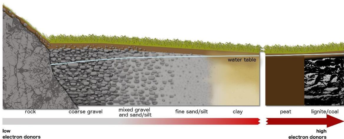
**Figure 46. Process-attribute gradient for soil types and redox.**
