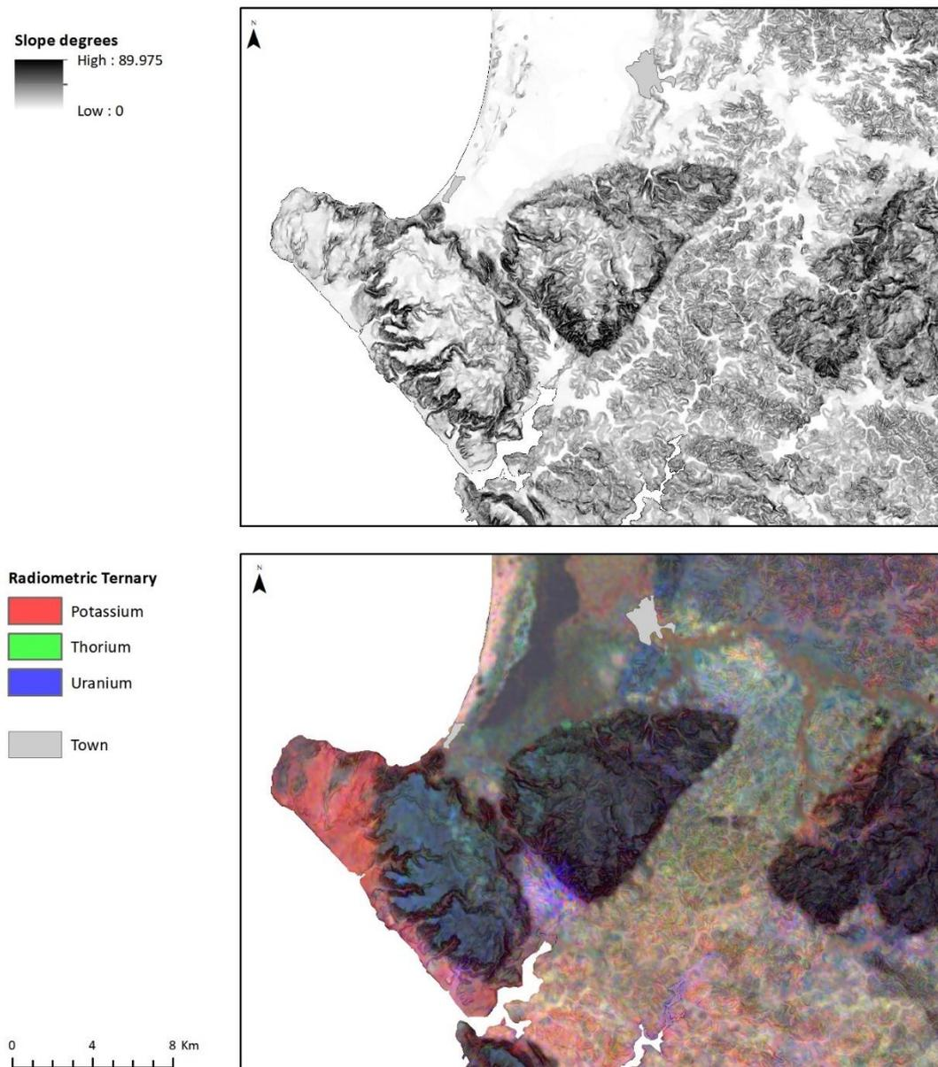
Figure 6. Ahipara test area comparison of radiometrics and DEM slope.
