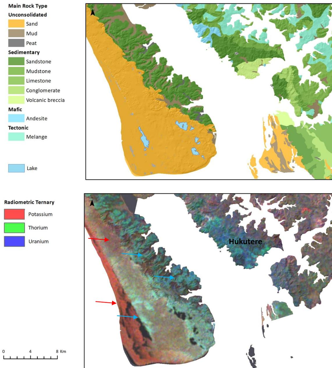
Figure 17. Dominant rock type from QMAP and radiometric ternary at Kaipara. Red arrows denote K-rich beach sands and beach sand derived sediments and blue arrows denote mantling by aeolian silt and clay.
