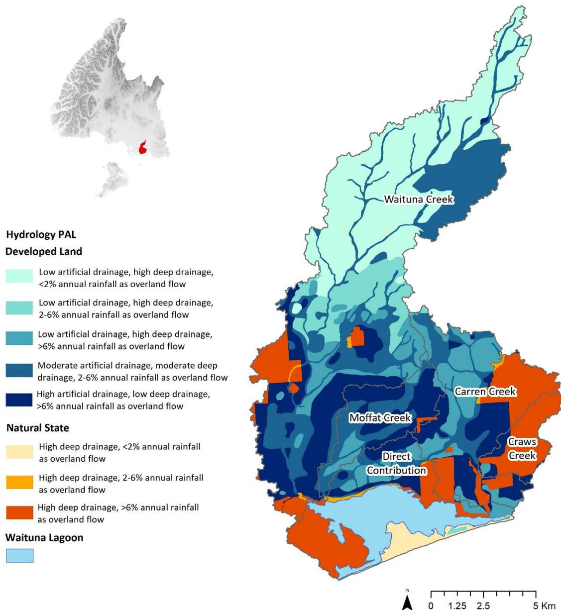
**Figure 45. Classed hydrological process attribute layer for Waituna Catchment intersected with fine scale flow paths of overland flow, deep drainage, and artificial drainage density.**
