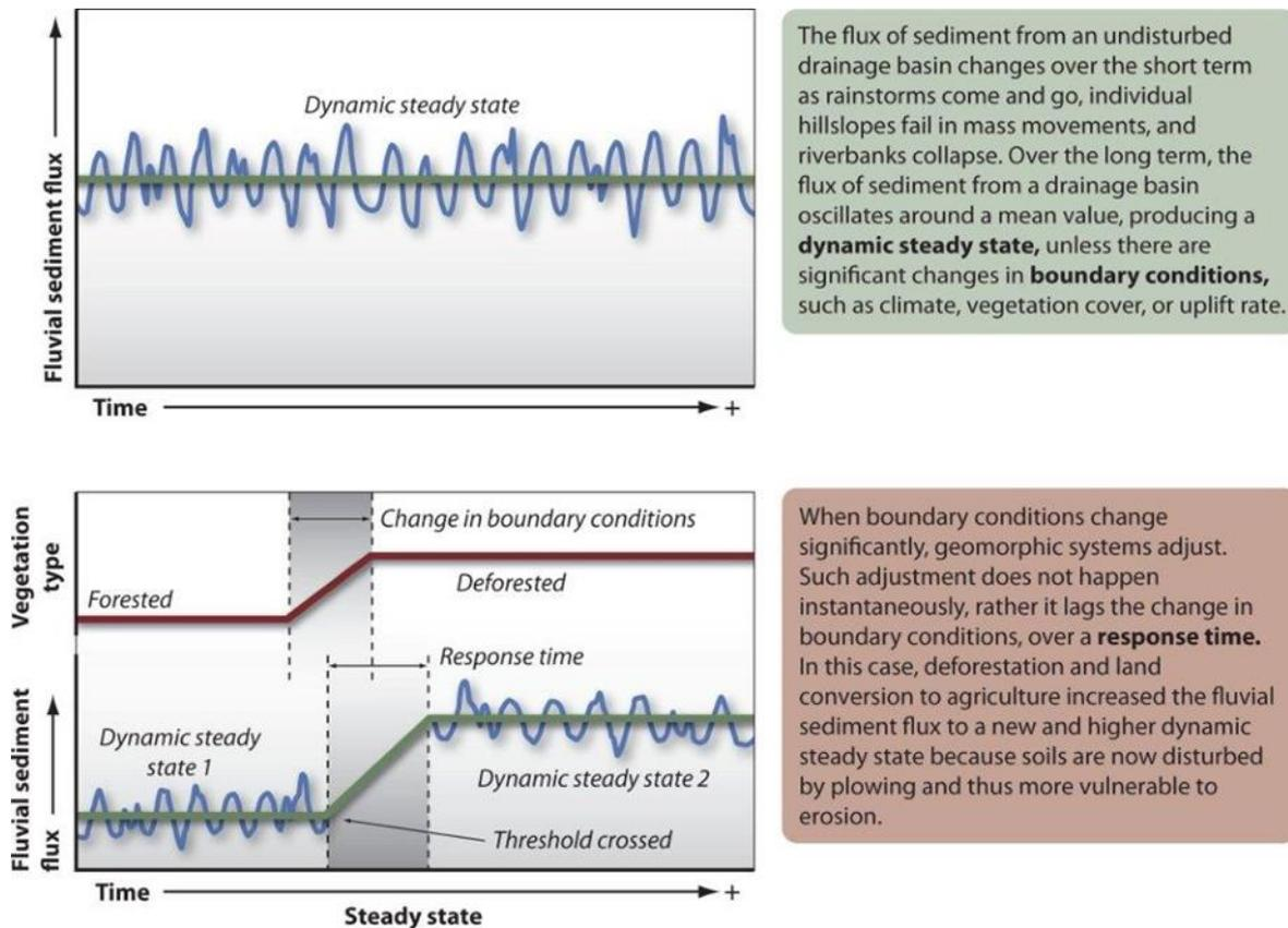
Figure 43. Proposed conceptual control over enhanced sediment loss from transport limited settings across Northland. Diagram from Bierman & Montgomery, "Key Concepts in Geomorphology, (2013)". Where the bottom text box refers to ploughing we redefine this as any activity that has significantly modified the hydrological response of the land surface.
