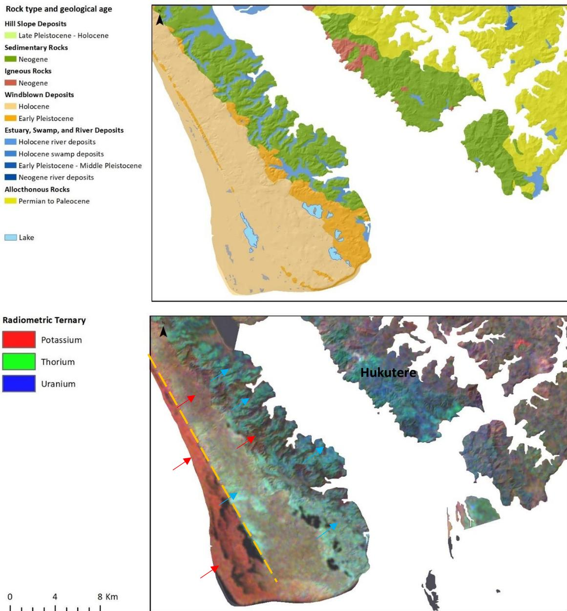
Figure 20. Rock type and age from QMAP and radiometric ternary at Kaipara. The blue arrows denote mantling by windblown silt and clay and red arrows show areas with K-rich sand.
