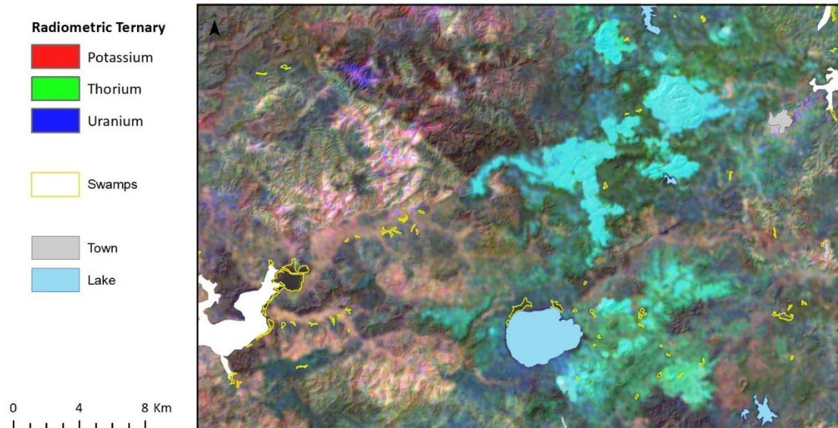
Figure 37. Swamps outline from LINZ and radiometric ternary at Waipapa. Gamma attenuation rates are high in areas of elevated water table (swamps). Drainage of swamps and subsequent soil evolution results in higher gamma values.
