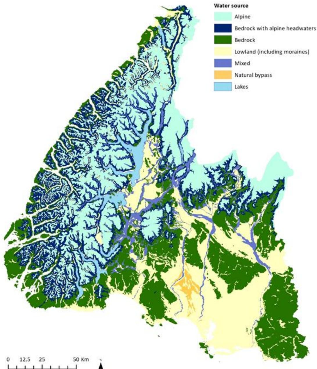
Figure 44. Classed process attribute layer for Southland hydrology (H-PAL). For clarity, overland flow layer and stream sources are not shown here. Where the map represents a classed process attribute layer which is classified according to hydrological tracers.
