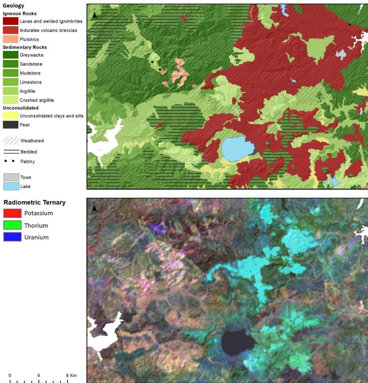
Figure 22. Rock type and transformation (LRI Rock2) and radiometric ternary at Waipapa.
