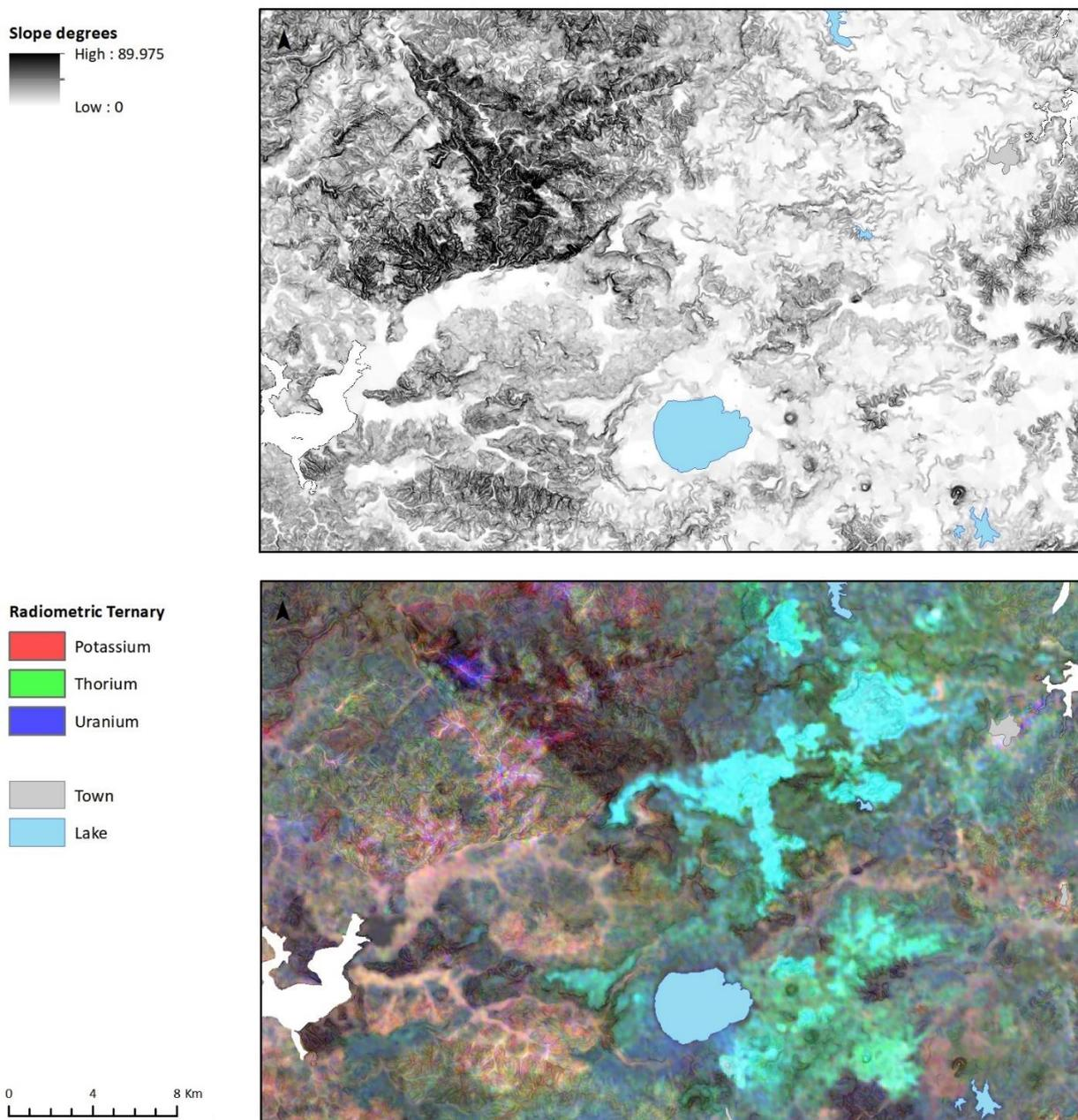
Figure 7. Waipapa test area comparison of radiometrics and DEM slope.
