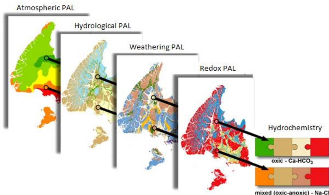
**Figure 48.** Conceptual diagram of how individual Physiographic Units that govern water quality were identified for the Southland Region. Areas with a similar PAL class assemblage for each PAL host similar process level controls and as such generate similar water composition.
