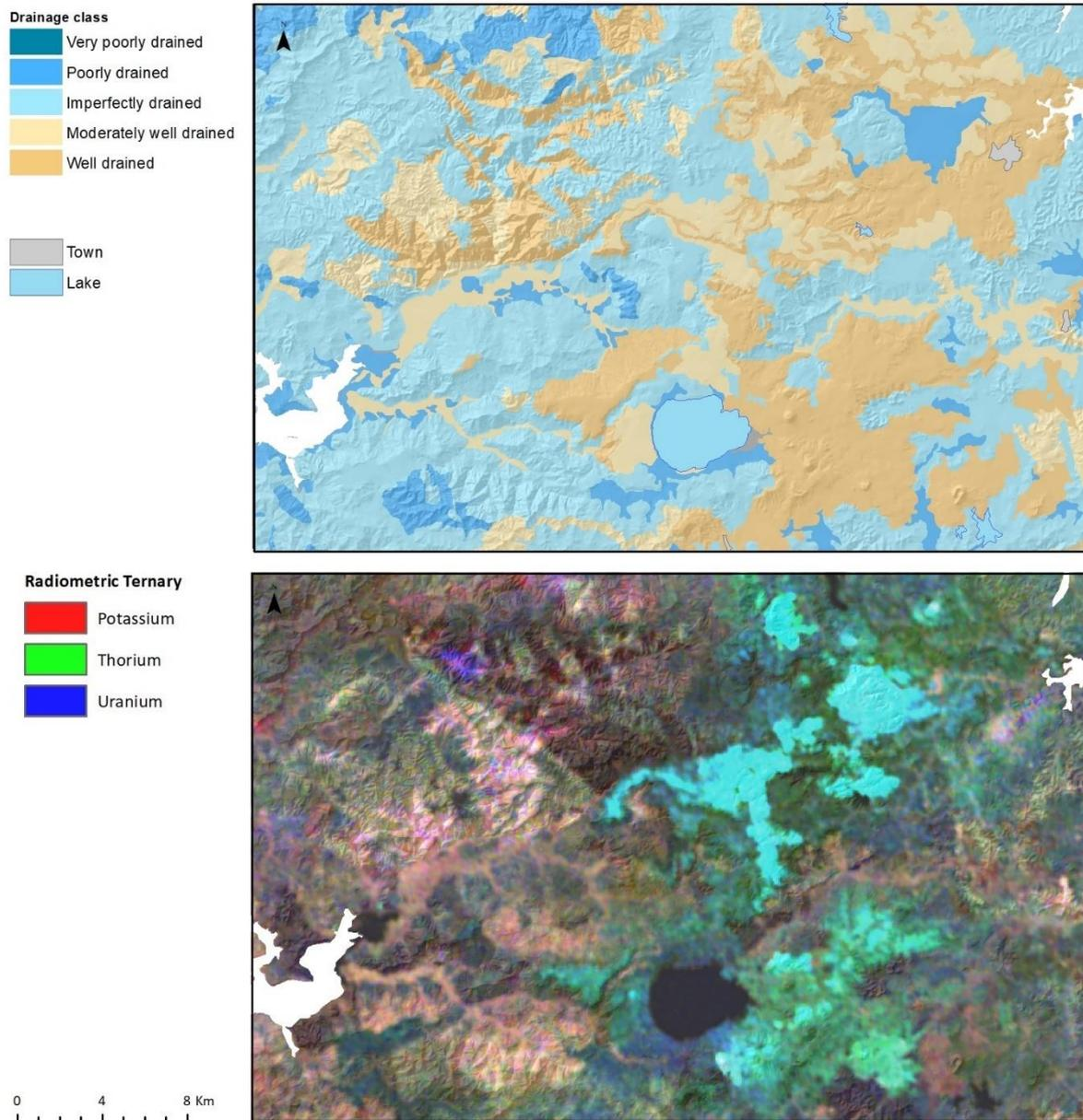
Figure 34. Drainage class from FSL and radiometric ternary at Waipapa.
