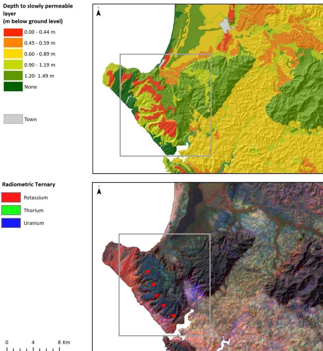
Figure 30. Depth to a slowly permeable horizon at Ahipara. The grey rectangle outlining some of the areas with finer-scale variation in landscape properties that do not appear to be well represented by the LRI. Red arrows in the radiometric ternary image denote intercalations of K-rich dune sand that has been blown along low lying valleys, which are not reflected in the LRI mapping.
